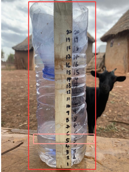
Figure 5: Rain gauge and surface detection
