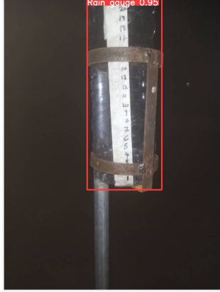
Figure 12: Illustration of accurate identification of the rain gauge even during nighttime
