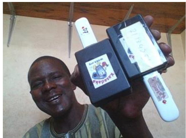
Figure 2. Adama Tessougué of Radio Sikidolo shows the Kasadaka box on which the Foroba Blon voice service now runs with its Bambara language interface.
