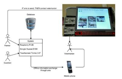
Kasadaka is a rapid prototyping platform build on a Raspberry Pi computer, designed to enable knowledge sharing between farmers and experts in rural developing areas across several domains. The Raspberry Pi is affordable, robust and easily replaceable, which makes it the ideal hardware to be used in this context. The software is open source and enables voice-based interaction, enabling illiterate, marginalized people to make use of the system.
